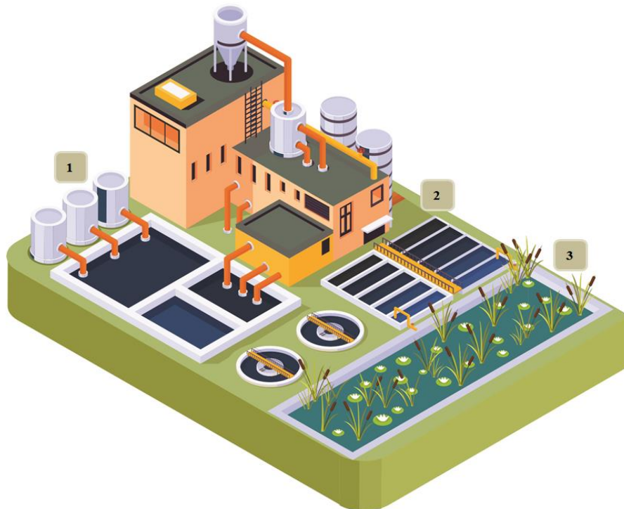
Figure 4. Water treatment process model in constructed wetlands. 1- Primary treatment. 2- Secondary treatment. 3- Tertiary treatment.
