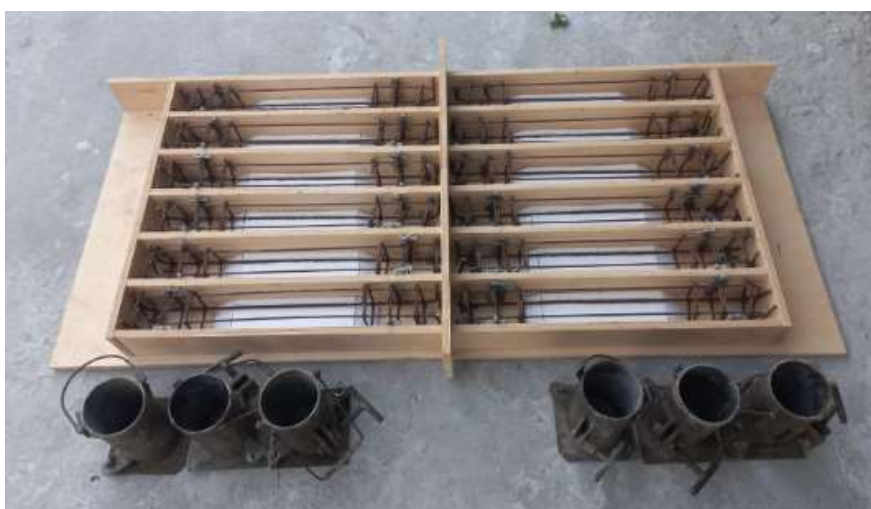
Figura 45 - Fôrma das vigas com as ferragens.
