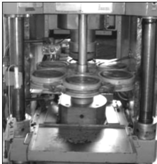
Figura 3.8 - Prensa industrial de 630 toneladas (BORGES, 2007)
