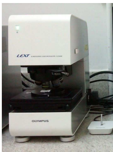
Figura 48 – Microscópio Confocal Olympus LEXT- 3D Measuring L Microscope 4000, do LAMAV/UENF.
