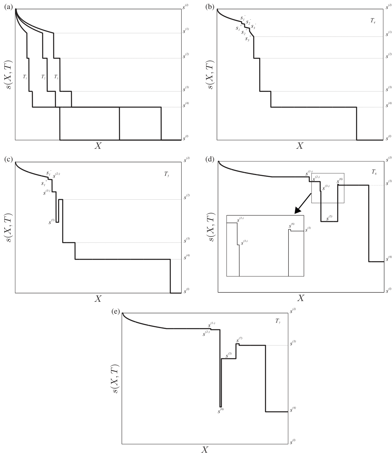
FIGURE 10 (a) Saturation profile for T < 1 ; (b) saturation profile when 1 < T < T_A ; (c) saturation profile when T_A < T < T_B ; (d) saturation profile when T_B < T < T_C ; (e) saturation profile when T > T_C
