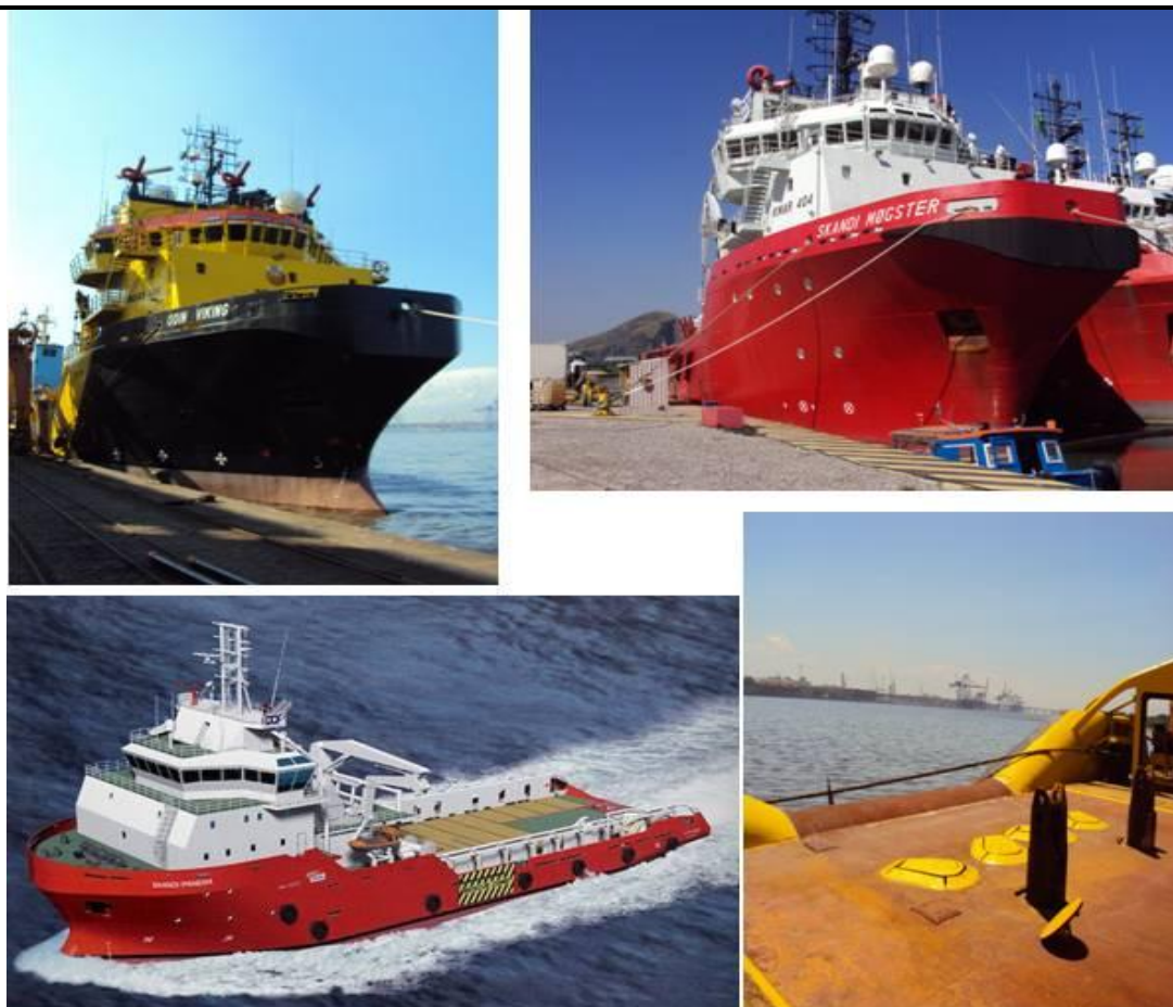
Figura 10 – Anchor Handling Tug Supply (AHTS) – Vistas laterais e shark jaw .
