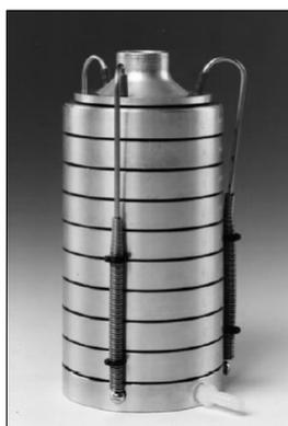
**Figura 14:** Aparelho de coleta de ar - Eight Stage Non-Viable Impactor.
