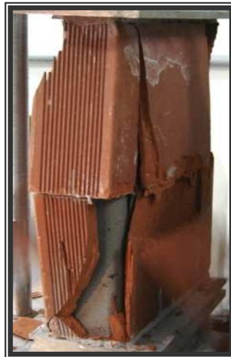
Figura 5.28 - Ruptura do groute
