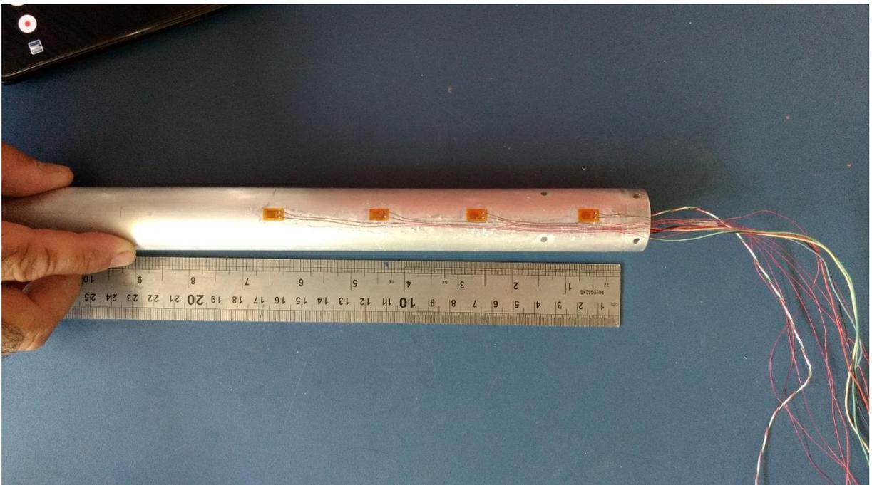
Figura 3.9 – Strain gauges.
