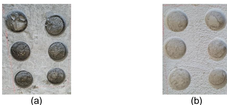
Figura 4.7: Ruptura das argamassas - (a) AD100; (b) AC100.
