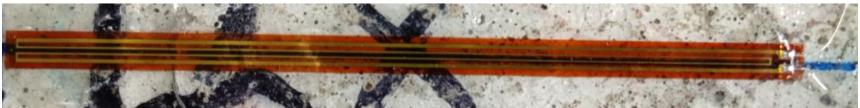
Figura 47 – Strain gage – Tipo 2 – BF120-100AA.
