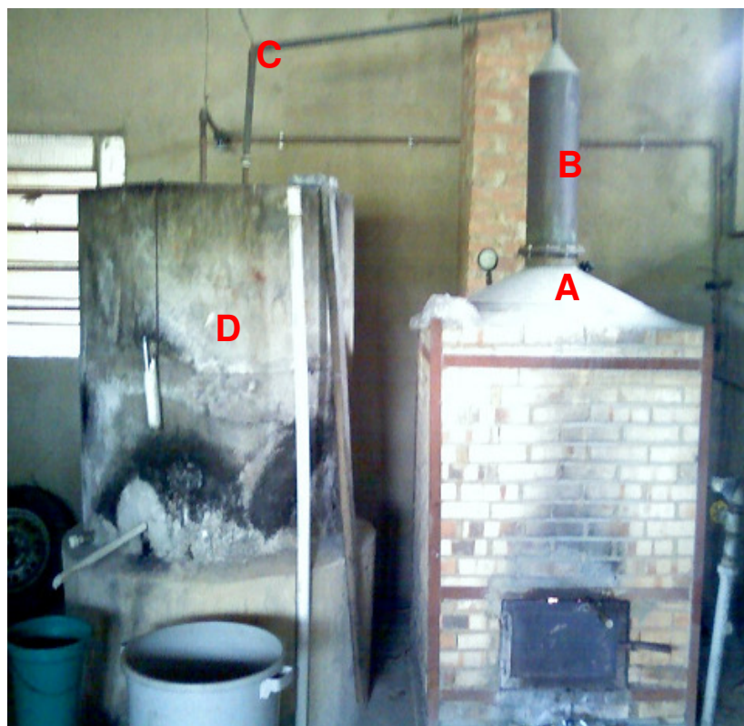
Figura 2 - Alambique 2. Legenda: (A) panela, (B) coluna, (C) alonga, (D) condensador.
