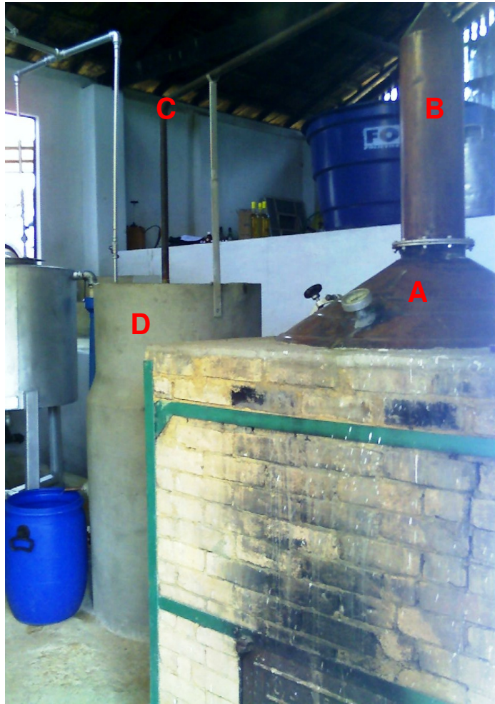
Figura 3 - Alambique 3. Legenda: (A) panela, (B) coluna, (C) alonga, (D) condensador.
